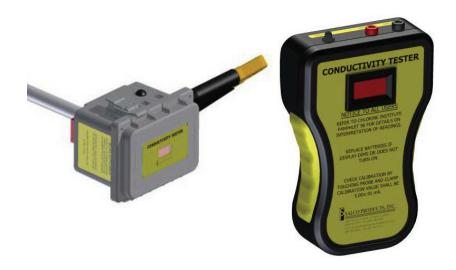
Salco Products conductivity tester has been designed for testing the integrity of rubber linings in railcars and trucks per Chlorine Institutes Pamphlet 98. The tester uses two 9V batteries and is rated from -25°F to 160°F. See Pamphlet 98 for acceptable commodities and concentrations that are acceptable for Milliamp Conductivity Testing.
